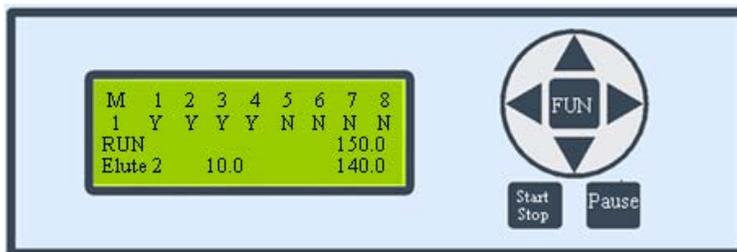
The screen indicates samples 1 to 4 are being processed using method 1. The total volume per sample is 150.0 mL and 140 mL has been processed. Currently the instrument is running the step of elution using solvent 2.
